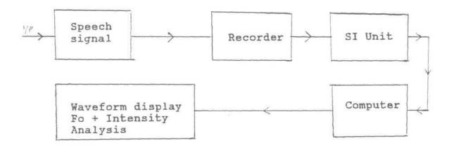
Fig: Block diagram showing the arrangement of instruments for the purpose of recording and analysis of speech.
