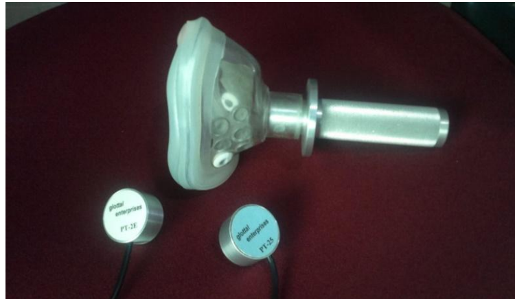
Figure 13: Aeroview mask along with pressure and airflow transducers.
