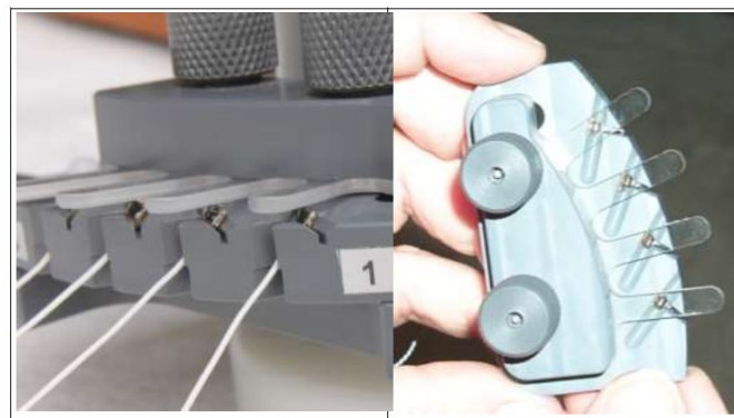
Figure 2. Mounted sensors inside the Magazine of Articulograph AG501
