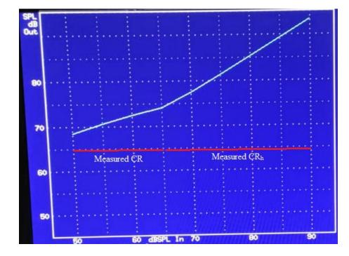
Illustration of measured CR and measured CR<sub>h</sub>
