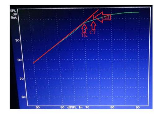
Illustration of computation of measured CT from the I/O graph
