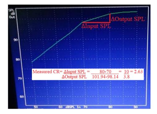
Illustration of computation of measured CR from the I/O graph
