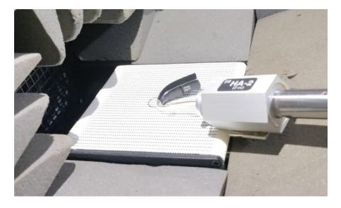
Setup of hearing aid in the FONIX 8000 sound chamber
