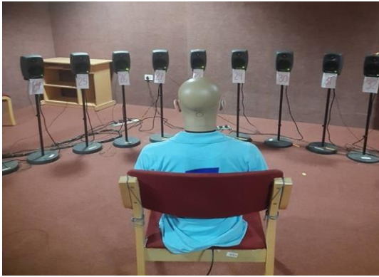
Figure 3.5: Kemar facing the loudspeaker, and the hearing aid was placed on Kemar right ear.
