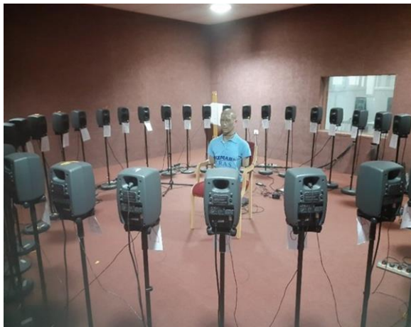
Figure 3.4: The Kemar facing the loudspeaker kept at a distance of 1 meter at 0 degree azimuth
