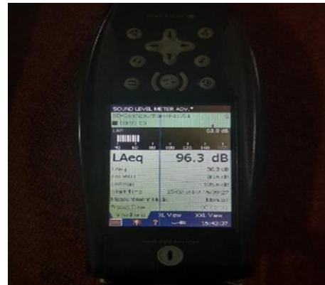
Figure 3.6: The Kemar was connected to the amplifier and the sound level meter (SLM) and the right panel showed the output level.
