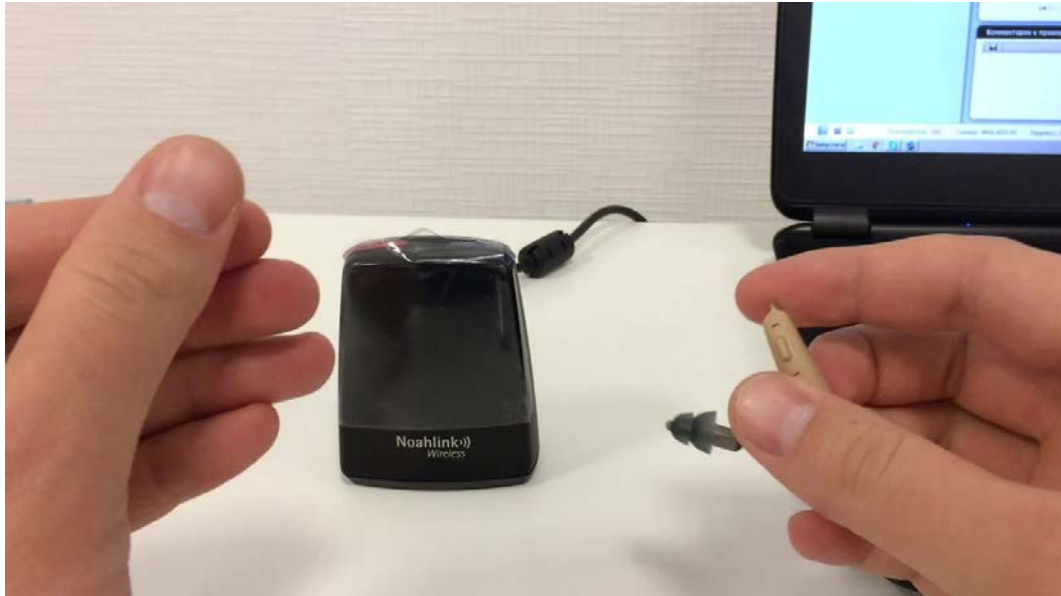
Fig 3.4. The digital hearing aid was connected through a NOAH link wireless to the Personal Computer (PC) with the software for programming the hearing aid.
