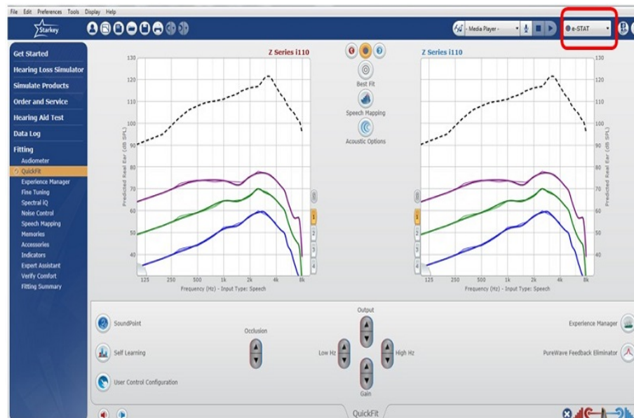
Fig 3.5. Programming the hearing aid by selecting the specific prescriptive formula. In the fig, the company specific fit for Starkey hearing aid using e-STAT software is show.
