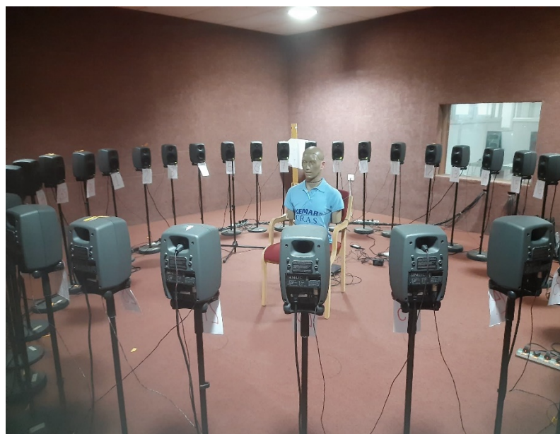
Fig 3.1. The setup for calibration, unaided and aided recordings. KEMAR was kept at 0-degree azimuth at a distance of 1 meter from the loudspeakers.
