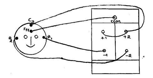
The above diagram illustrates how the electrodes were placed and how they were plugged into the electrode head box.
