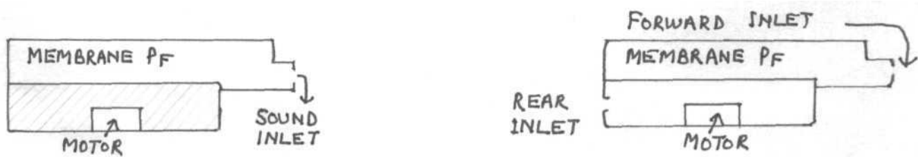
Fig. 2-8: P_F ( Pressure in the Forward Inlet ) P_R ( Pressure in the Rear Inlet )
