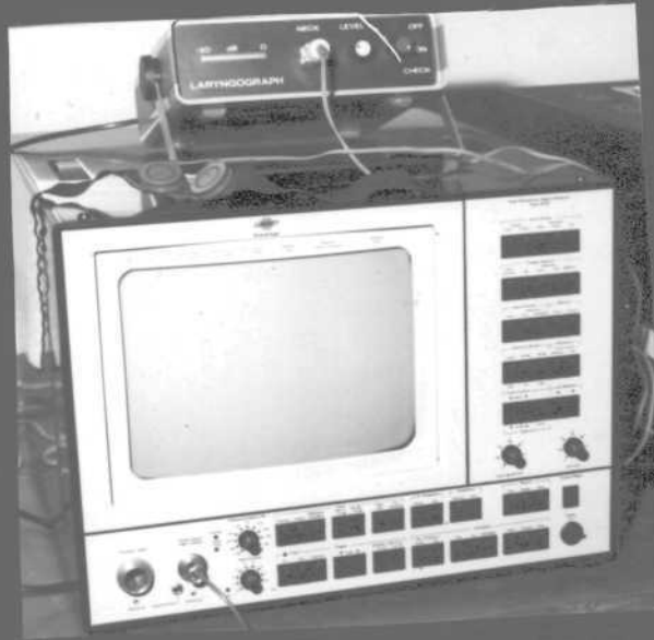
Photograph-1: High Resolution Signal Analyzer with Laryngograph.
