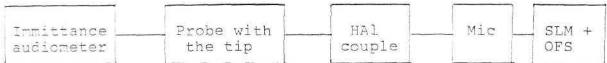
Figure 8: Block diagram of instruments for the calibration of output SPL of immittance audiometer
