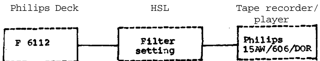
Fig.(c) The instrument set-up for the filtering process.
