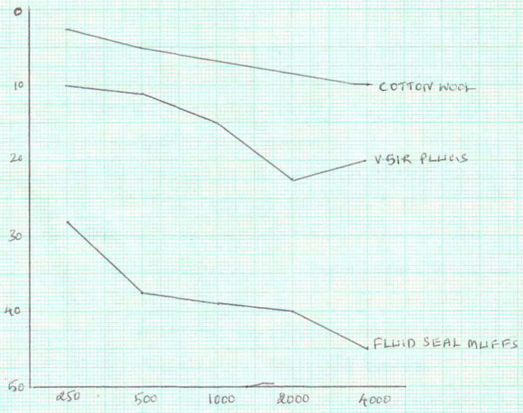
Figure 1. Average Sound attenuation values of various Ear protectors.
