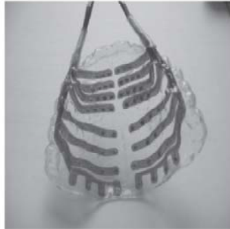
Figure 2. 2, A pseudopalate containing 64 electrodes that record tongue palate
