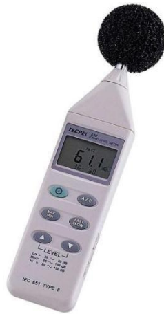
Figure 4: Sound Level Meter (TECPEL DSL-331).
