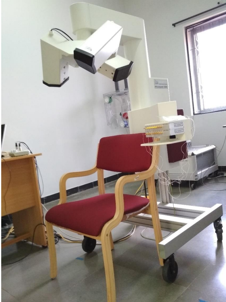
Figure 1: Showing calibrated instrumental setup of AG 501.
