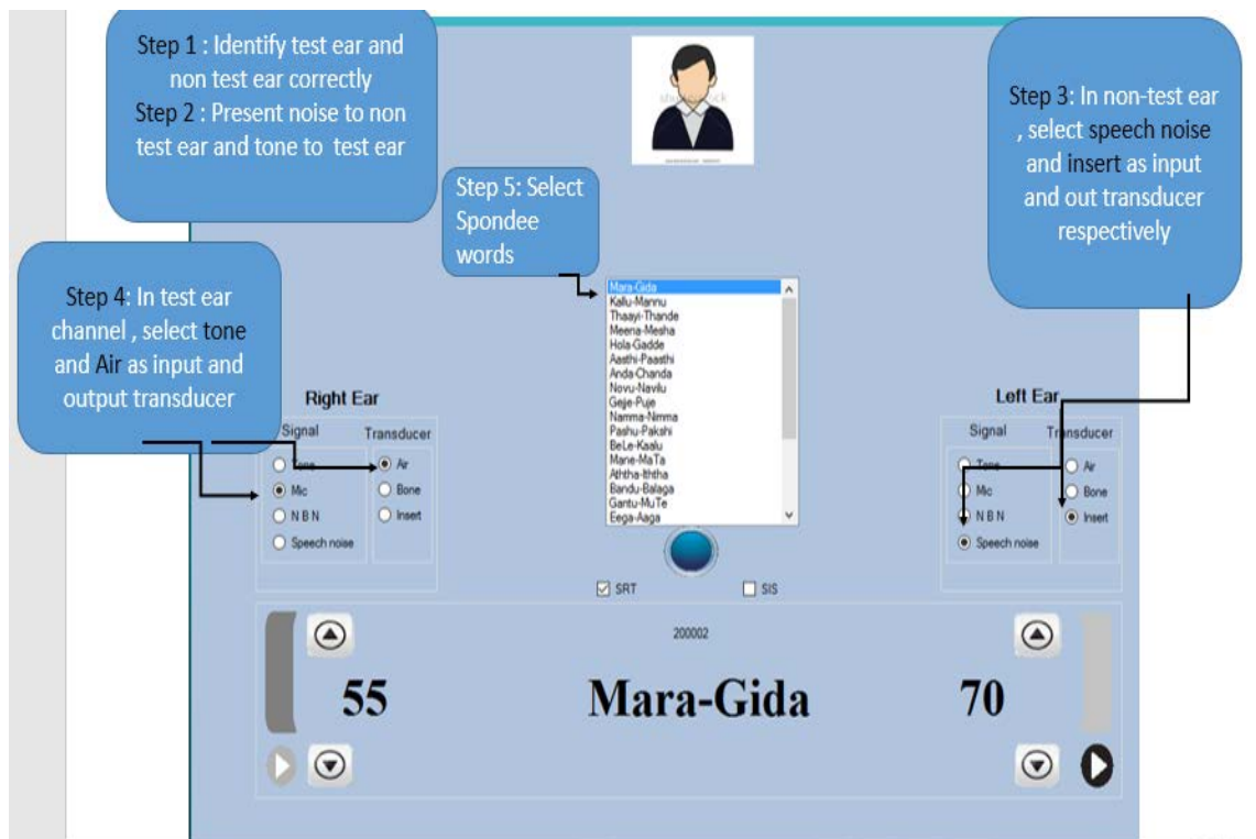
Figure 2. 8. Represent SRT masking in speech audiometry module in the software.
