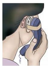
b. Add-on amplifier: This type of amplifier can be attached to the receiver end of the existing telephone. It can be removed from the telephone. The biggest advantage of this amplifier is that it can be used with different phones. The user may even carry the add-on amplifier around and use it when he/she uses public/other phones. These amplifiers are also cheaper and easy-to-use. However, they may not work with all phones. Also, batteries need to be changed regularly.
