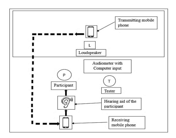
Initially, the aided performance of the RIC hearing aid with microphone input, without a mobile phone, i.e., through the loudspeaker of the audiometer, was measured in
