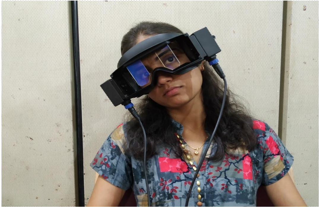
Figure 3.2: Subject at right thirty-degree head position wearing binocular VNG goggles.
