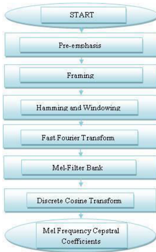
Figure 4: Mel Frequency Cepstral Coefficient Block diagram.
