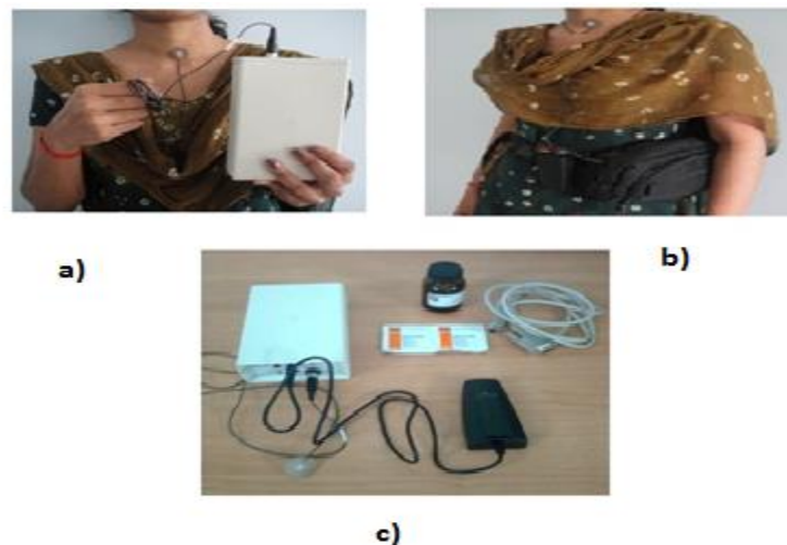
Figure 3.1. Ambulatory Phonation Monitor (APM) gadget a) connection between throat sensor and APM hardware module; b) APM has worn by a participant in the waist pack. c) APM- hardware module, throat sensor, Vibro- tactile unit, adhesive glue and glue remover, PC connector.
