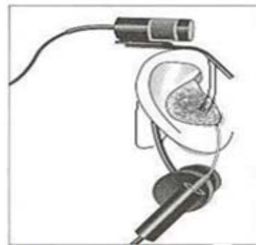
Location of the reference microphone and probe tube microphone along with hearing aid for REAR
