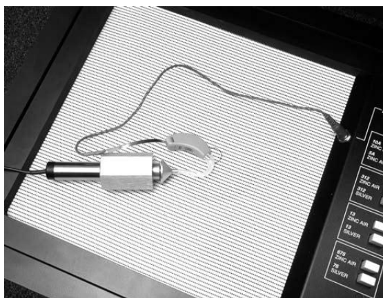
Figure 3.6. The output of hearing aid, being picked up by the microphone through the coupler and adapter. This is fed to Fonix 7000 hearing aid analyzer for electroacoustic measurement (Reprinted with permission from Frye electronics, Inc.).
