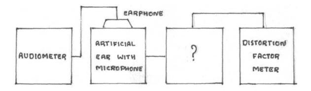
3. Pure-tone total harmonic distortion measurement using sound level meter with octave filter set requires
