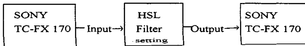
Fig.B Instrumentation set-up for filtering process
