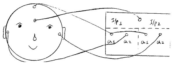
The above diagram illustrates the placement of the electrodes and their connection to the electrode box. After the electrode was placed, the impedance was checked. If the impedance was within the specified limits, the earphones were placed without dislodging the electrodes (Blue-left ear; red-right ear).
