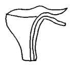
1/2 shell: In between a semiskeleton and canal lock. Excellent retention if patient has ears which are tender or comprised of hard cartilage.
