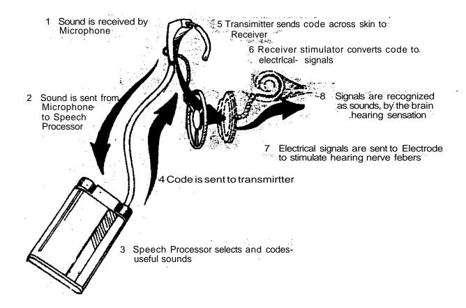
The microphone picks up the sound changes it into small electric current and sends it to the signal processor. The signal processor modifies the electric current. The electric current is sent by way of a cord to the external coil and changed to a magnitic field. When the external coil is held over the internal coil, the magnetic field causes the current to flow through the internal coil and the electrodes. The electric current "stimulates" the hearing nerve.
