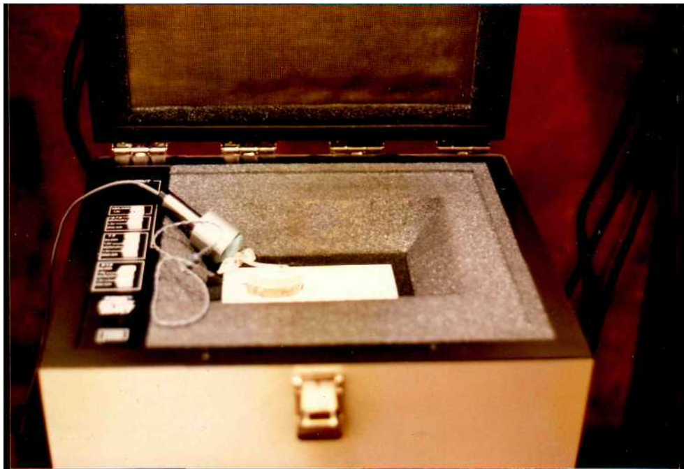
Photograph 1. Showing connections within the hearing aid test system.
