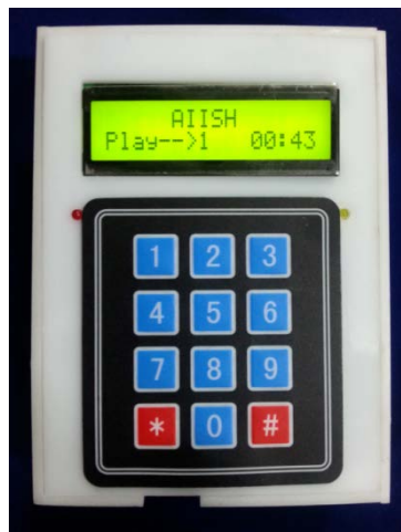
c. Screen showing the code no. of the exhibit of which the commentary is being played
