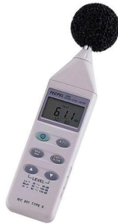
Figure 4: Sound Level Meter (TECPEL DSL-331).
