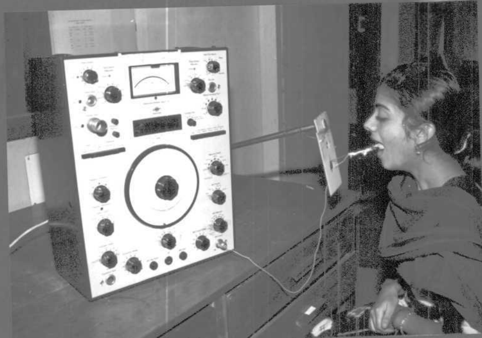
Photograph showing the instrumentation used for measuring optimum frequency (Hetro dyne analyser)
