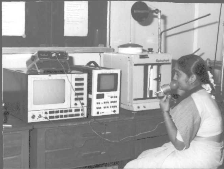
Photograph-1: Measurement of MAF rate and Electroglottograms simultaneously
