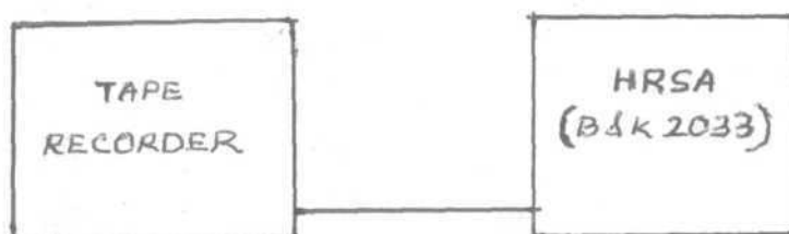
Fig.3.5: Experimental set up for the measurement of vowel duration.
