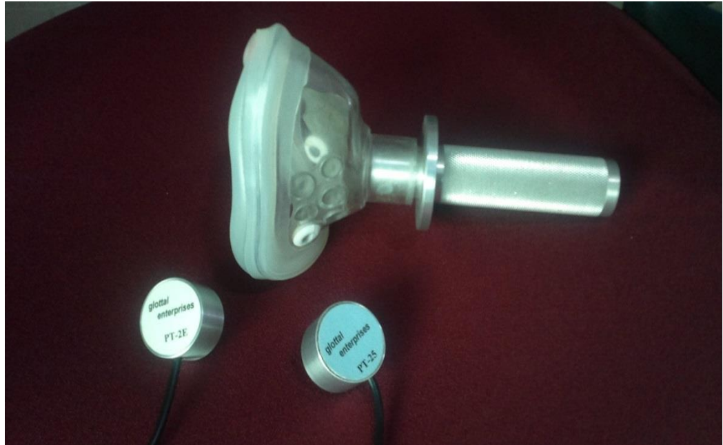
Figure 2. Pneumotachograph mask with PT-2E wideband airflow transducer and PT-25B pressure transducer.
