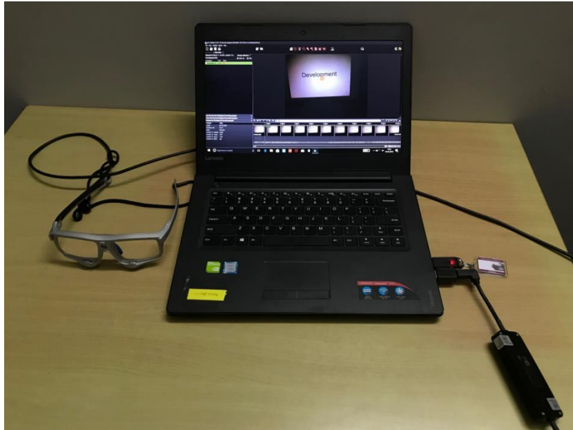
Figure 3.1: SMI Eye tracking instrument set- up for the experiment
