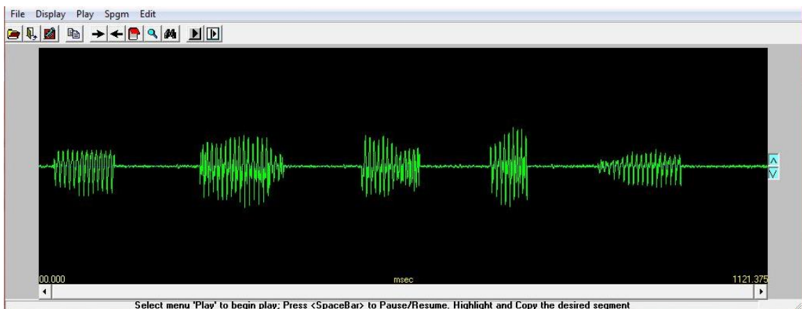
Figure 15: Depiction of segmentation window showing 5 occurrence of /m/ for a speaker.
