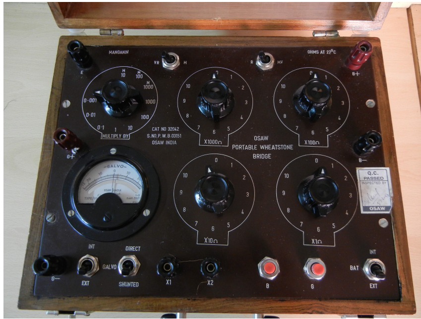
Figure 1.2: A wheatstone bridge setup.
