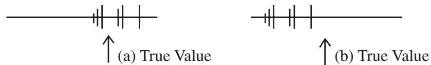
Fig 1: Set of results (a) without systematic error and (b) with a systematic error.
