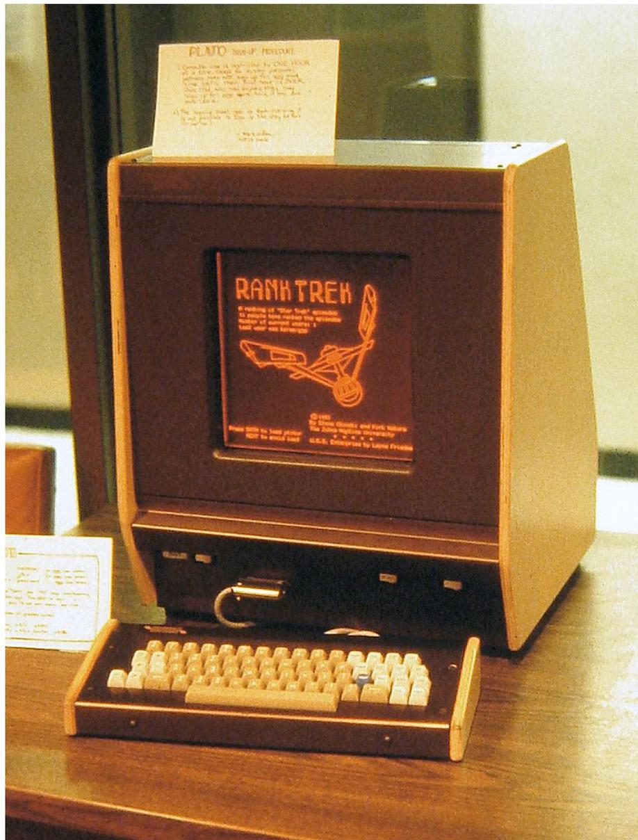
wired to interpret only a limited number of simple control codes, without any programmability and local computing capabilities. The PLATO V terminal, on the other hand, was based on an Intel 8080 microprocessor [169] and was thus able to execute programs downloaded from the host computer—this is very similar to how today’s Web browsers execute ECMAScript (JavaScript) code downloaded from a Web server.
