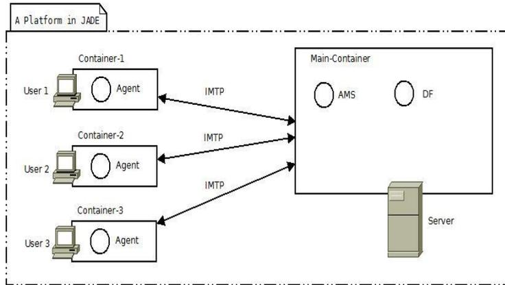
Figure 1. A platform with multiple containers
