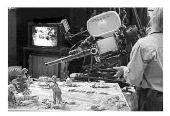
In the photo on the right, the camera operator uses a lens probe to film a miniature prehistoric setting that will later come to life in a full-scale effect. Although this is a film camera, it has a video viewfinder to provide immediate feedback on the image captured on film. (Note the video monitor).
