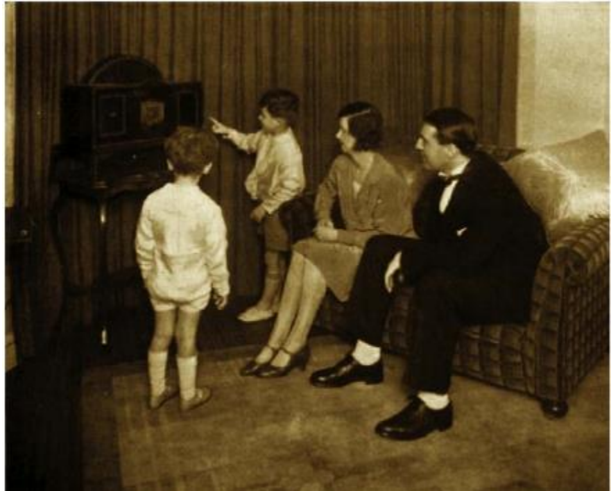
FIG. 1.1 British family watching a 1930 Baird Televisor, a mechanical scanning TV. Courtesy MZTV Museum.
