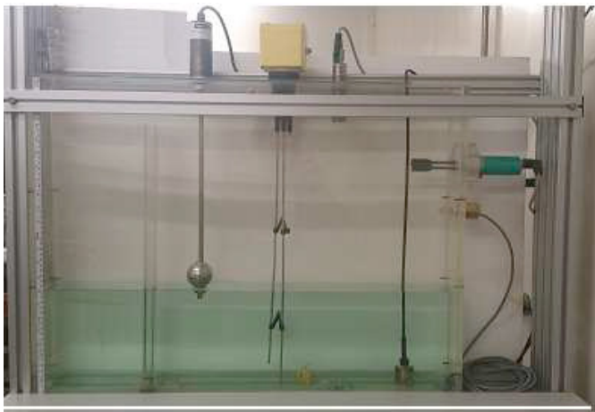
Fig. 1. Level transmitters and detectors workbench.
