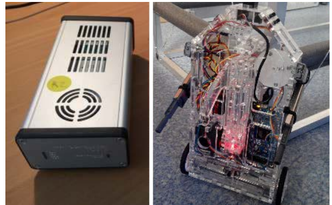
Fig. 1. Thermo-optical system (TOS1A) and Segway laboratory model.
