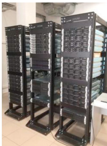
Fig. 5. Multicomputer system (cluster) for parallel and distributed computing and data storage.
