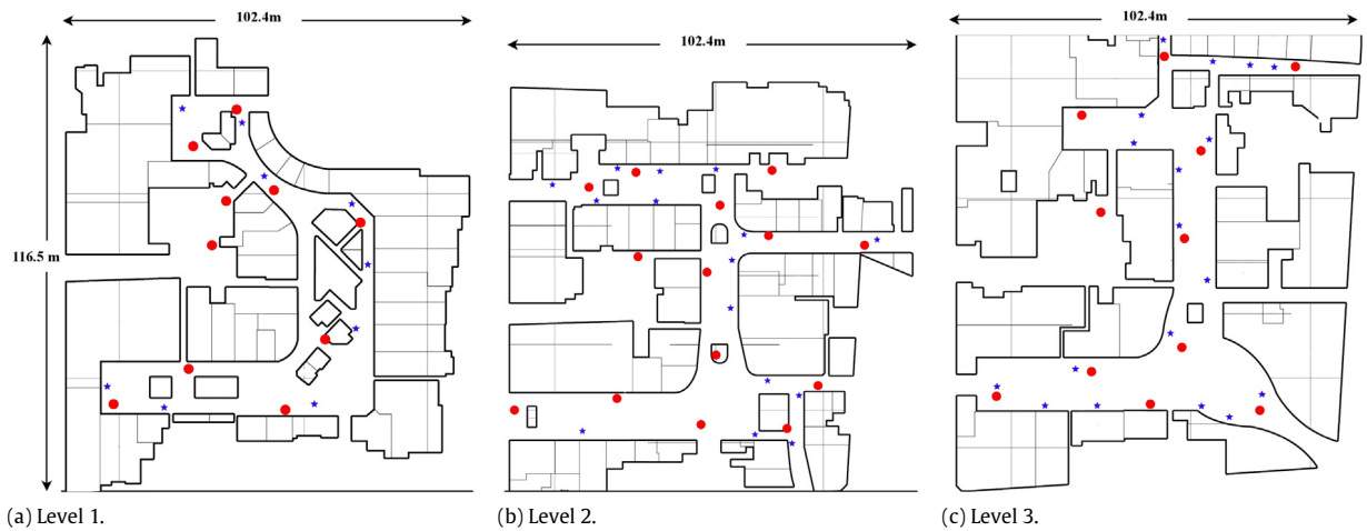
Fig. 6. The floor maps in the mall where the experiments are conducted. The red dots represent the Wi-Fi APs, and the blue stars denote the test locations where ground-truth RSSI information were collected. (For interpretation of the references to color in this figure legend, the reader is referred to the web version of this article.)
