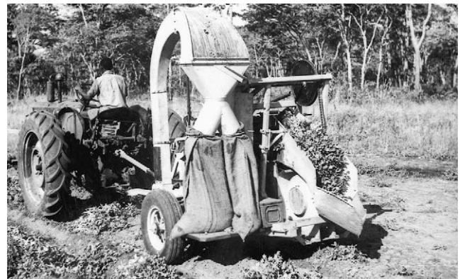
Figure 2.3 – Groundnut harvester at work in Tanganyika – development started in the 1950s.
