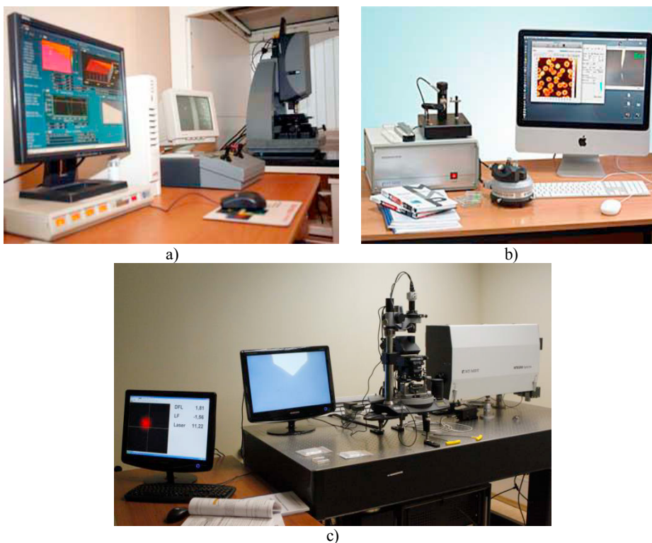
Fig. 4. Measurement equipment: a) 3D imaging surface structure analyzer NewView 5000; b) high-speed camera VS-FAST/C/G6; c) scanning probe nanolaboratory Ntegra Spectra.
