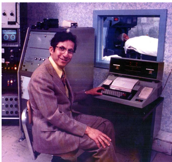
Fig. 1. Robert Ledley at the control console of the first whole-body CAT scanner, Georgetown University, circa 1974.
